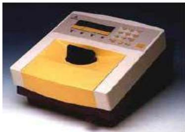
The Triathler's portable liquid scintillation counter is a very compact system. This can be used for in-situ estimation of beta emitters in water like Sr-90, H-3, S-35 etc.
